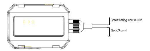
Figure 6. Typical Analog Input Connection
