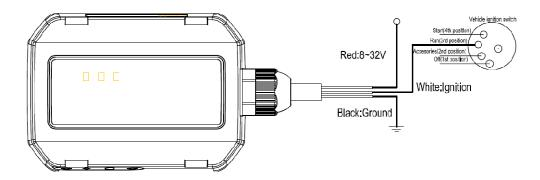
Figure 4. Typical Ignition Detection
