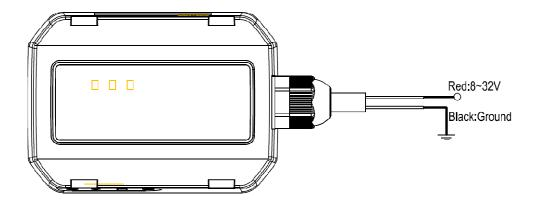
Figure 3. Typical Power Connection
