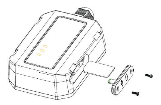
Figure 2. SIM Card Installation
