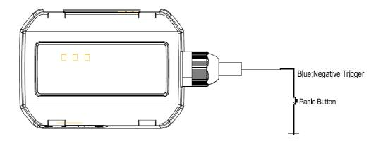
Figure 5. Typical Digital Input Connection
