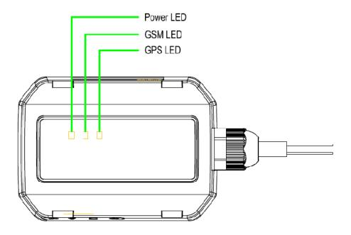
Figure 8. MT100 LED on the Case
